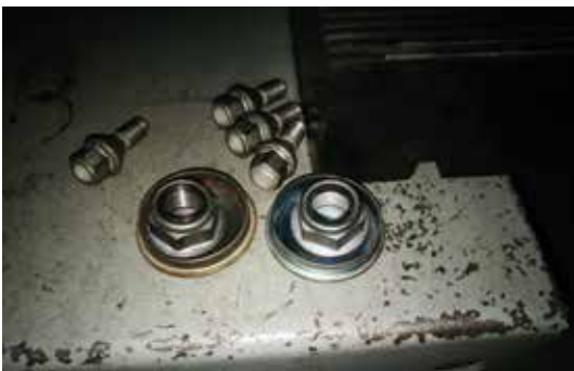
Example: Replacement of accessories (Fixing nuts, bolts and protective cap)
