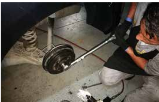
Example: Ensure the correct torque, according to manufacturer, using manual torque wrench
