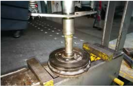
Example: Linearity between housing and bearing in installation (1st. Generation)
